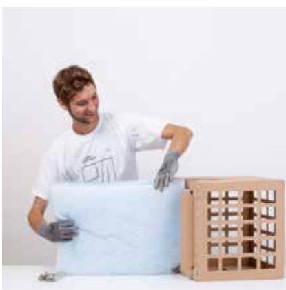
Step 2: The filter medium is inserted: Coloured side inside, and exact fit in the box.
