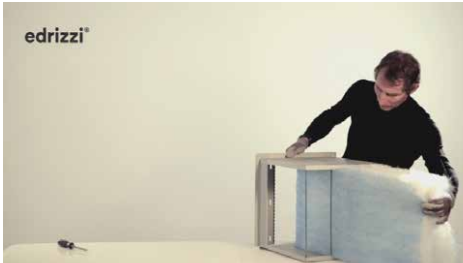
Step 1: To insert the filter medium, fold it exactly in the middle and pull it with the colour inside through the clamp in the frame.
