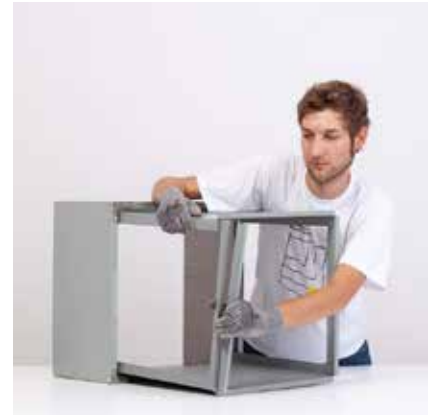
Step2: The brackets are fixed with rivets to the base.
