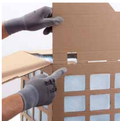
Step 3: The filter medium is fixed with a tackers, the straps at the top are latched for stability and the box is closed. The completely ready box is pushed into the holding frame.
