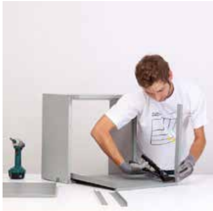
Step2: The brackets are fixed with rivets to the base.
