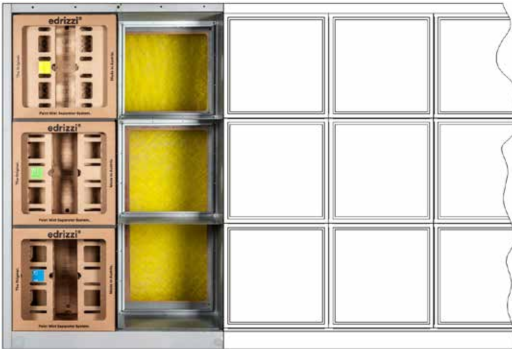
Figure: The correct installation of the edrizzi® paint mist separator in the slide-in elements for standing application.
