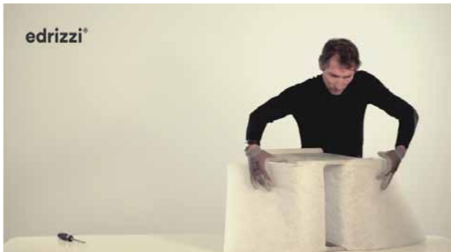
Step 2: The filter medium is disguised with the coloured side inside over the outer edges of the frame.
