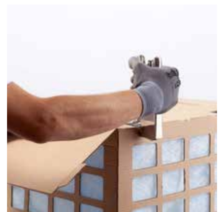
Step 3: The filter medium is fixed with a tackers, the straps at the top are latched for stability and the box is closed. The completely ready box is pushed into the holding frame.
