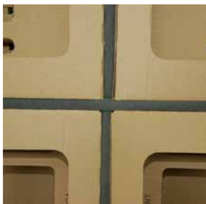
Figures: Left an adhesive tape and right a rubber band are used to seal off the paint mist separators.
