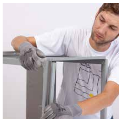
Step 5: Attention: Before the last bracket is fixed with rivets, hook the locking bar behind at the top and bottom of the holes provided for this purpose.
