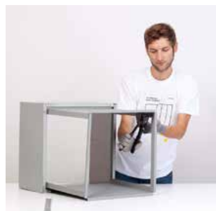
Step 3: The cover is pushed in and fixed with rivets to the upper end of one bracket.
