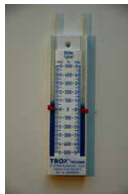
Example for a pressure gauge: The U-tube pressure gauge.
