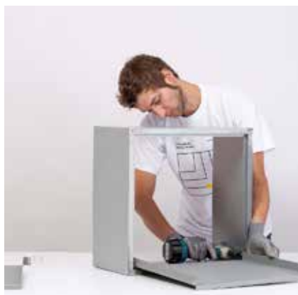
Step 1: The base is inserted and connected from inside to outside with self-tapping screws.
