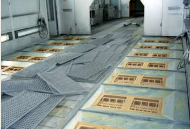
A Venturi scrubber system can be replaced by an Edrizzi dry filter system in only a few days
