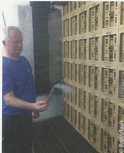
After control of the initial pressure difference and recommended inflow speed, the paint mist separation is ready for painting operation.
